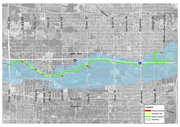
Figure 2. 100 Year Floodplain along the Little Calumet River near the Gary – North Levee
